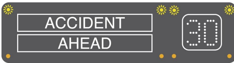
Temporary maximum speed advised and information message
